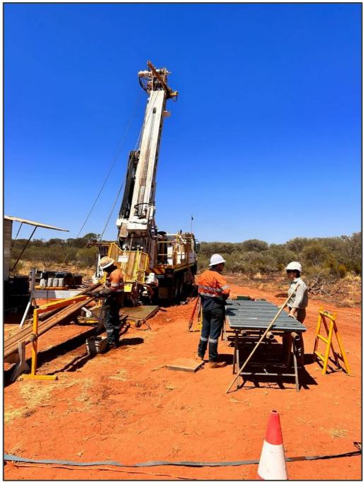
Figure 2: PX Drilling Rig drilling LEDD001
