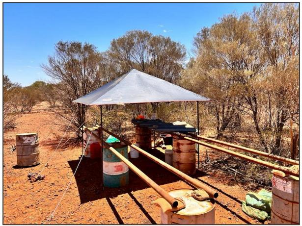
Figure 4: Remote exploration basic core yard set up allowing the team to process core on site.
