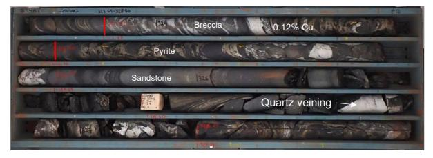
Figure 4: Core tray of LEDD002 showing the strong deformation of the stratigraphy.
