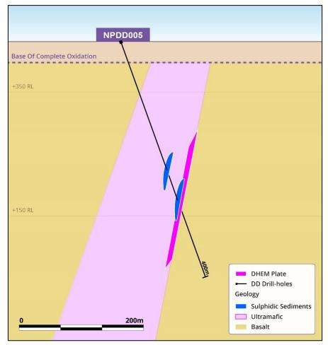
Figure 2 – Cross-section A – A' (see Figure 1) showing completed diamond drill-hole NPDD005 and the modelled DHEM conductor in relation to the modelled ultramafic unit, sulphidic sediments and interpreted footwall contact
