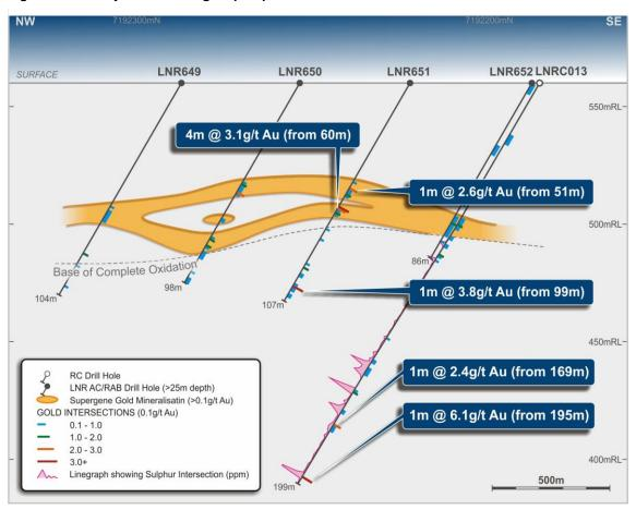
Figure 3 Drill section showing relationship between sulphur distribution (pyrite alteration) and gold mineralisation.
