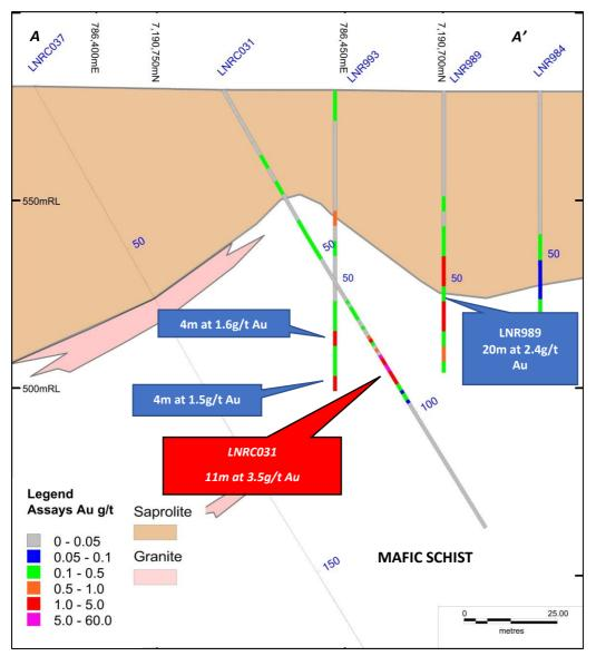
Figure 3. Gidgee Flat cross-section A-A' showing LNRC031 intersection.
