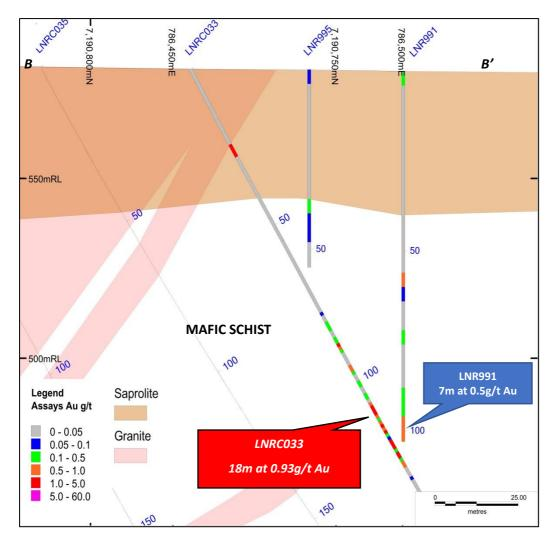
Figure 4. Gidgee Flat cross-section B-B', showing LNRC033 intersection.
