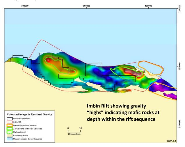
Figure 6 Gravity Image of the Imbin Rift
