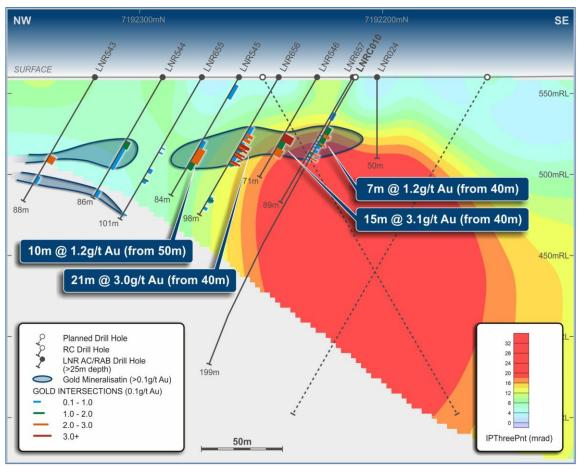
Figure 3 Section 69700N showing modelled IP chargeable target in relation to drilling, planned RC holes shown on section.
