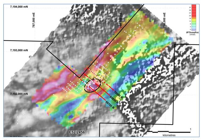
Figure 2 Gradient Array IP image overlying detailed 1VD magnetic image. Strong chargeability zone outlined in black, pole-dipole traverses shown as red lines and drill collars greater than 25m depth shown in white. MGA94 Zone 50
