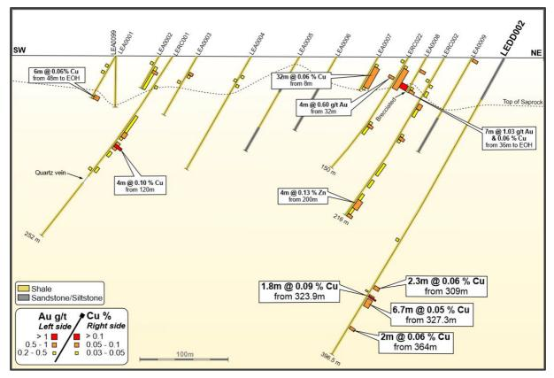
Figure 2: Drill cross section showing LEDD002 results and earlier aircore and RC drill intersections
