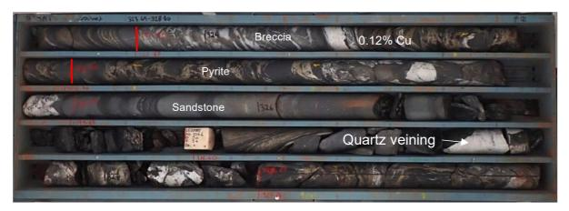
Figure 3: Core tray of LEDD002 showing the strong deformation of the stratigraphy.
