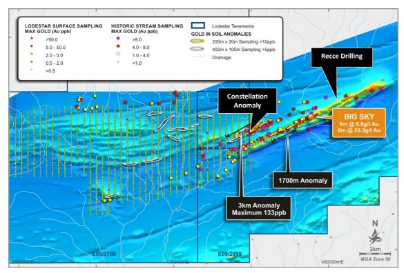
Figure 1 Gold anomalies and aircore drill targets, Camel Hills.
