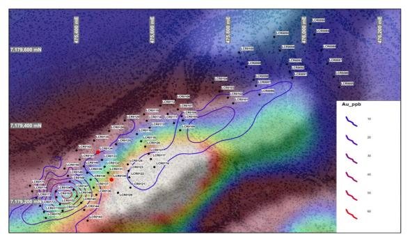
Figure 2 Drill hole location (anomalous drill holes highlighted in red), showing Constellation gold in soil contours on 1VDRTP magnetic image.
