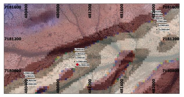
Figure 3 Reconnaissance drilling (anomaly highlighted in red) on 1VDRTP magnetic image.
