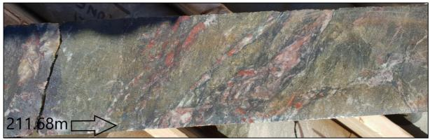
Image 1: diamond drill-core LND004, 211.68m (6.94 g/t Au) with Haematitic Syenite and pyritization
