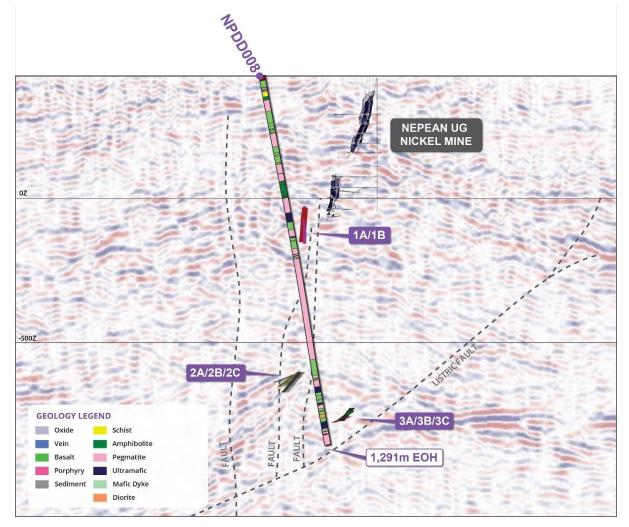
Figure 1 - Cross-section showing diamond hole NPDD008 drilled below the historic Nepean mine workings, showing multiple ultramafic units in dark blue and the modelled plates for the identified off-hole DHEM conductors. Background is the 2D seismic survey section with relevant interpreted structures.
