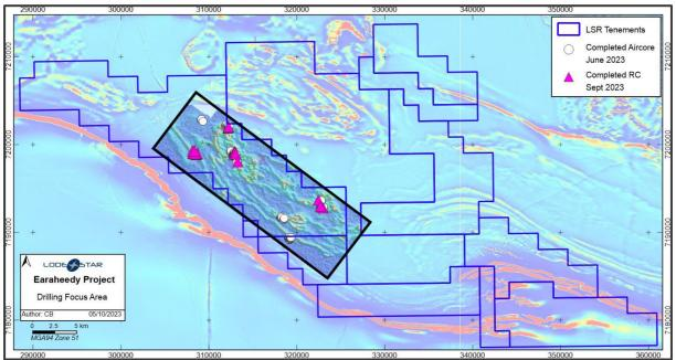
Figure 7: RC drill hole locations on magnetic background.
