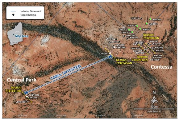
Figure 1 Drill hole location plan showing re-sampled drill holes (green dots) and 1m split samples for assay (white dots).
