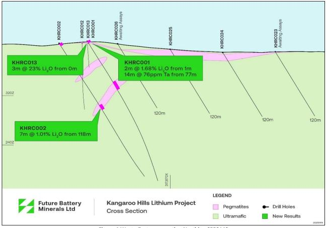
Figure 4:West - East cross section Northing 6558140
