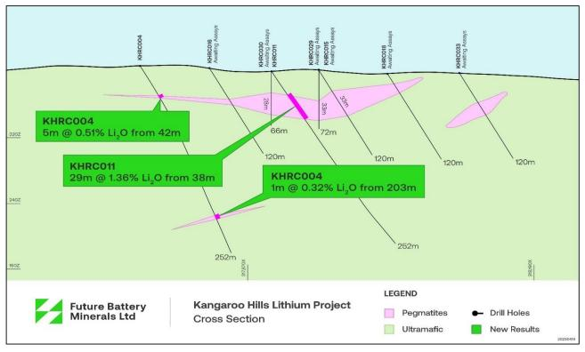
Figure 2 West- East Cross Section – Northing 6558300
