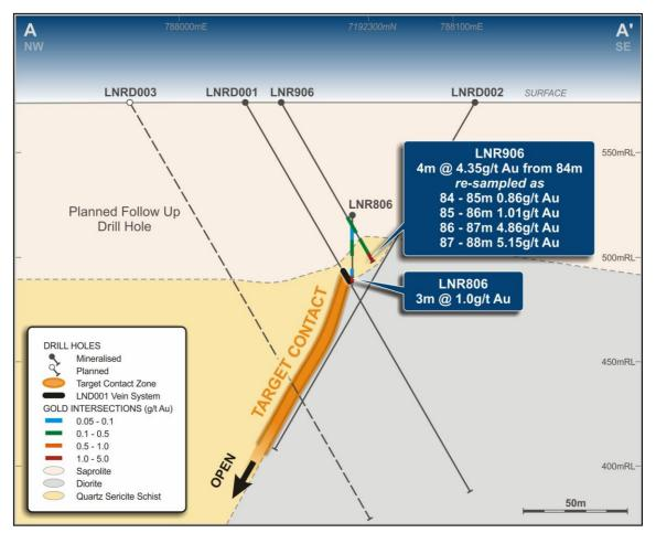
Figure 3 Cross section view of LND001 and interpreted geological contact, showing planned down-dip drill hole test.
