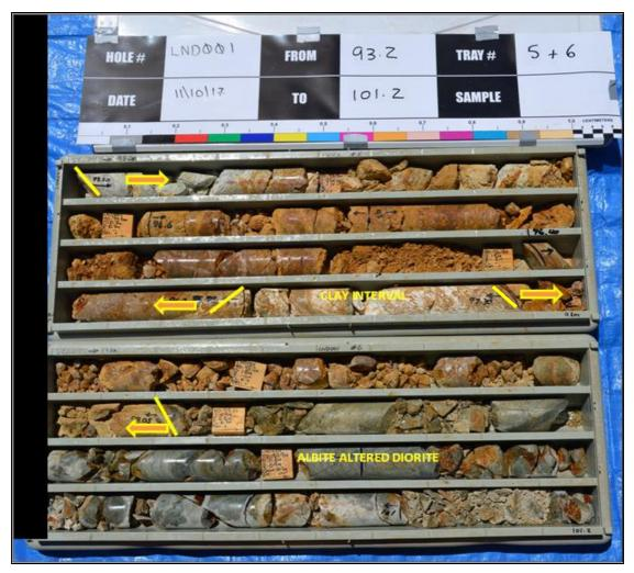
Figure 2 Brecciated and strongly ferruginous (brown) quartz vein system located on the contact between felsic schist and diorite. Vein interval is shown by the yellow arrows.
