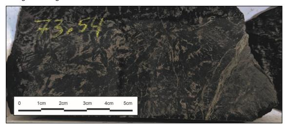
Photograph 1 – Section of half core from diamond drill-hole NPDD007 showing the distinctive net-textured "triangular ore zone" nickel sulphide mineralisation (4.06% Ni, 0.19% Cu)
