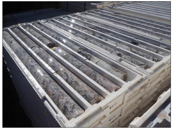
Photograph 1 – NPDD008: part of the thick pegmatite intrusion below the historic Nepean nickel mine from 641.5-993m. Interval shown starts at 663m down-hole
