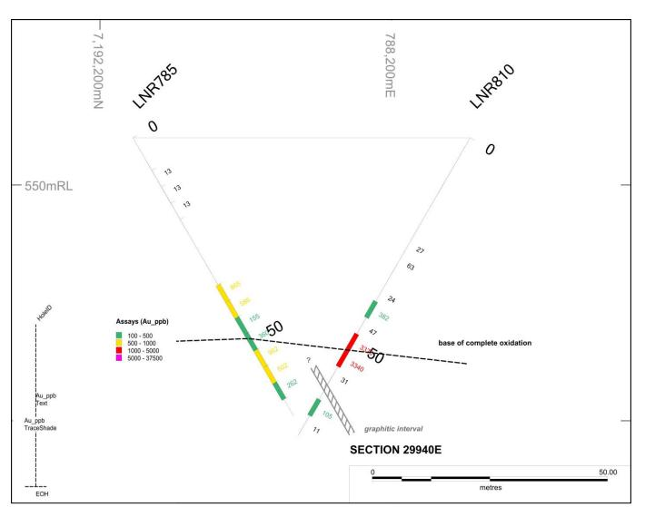
Figure 7 Contessa drill cross-section 29940E, looking northwest (gold assays greater than 10ppb Au).
