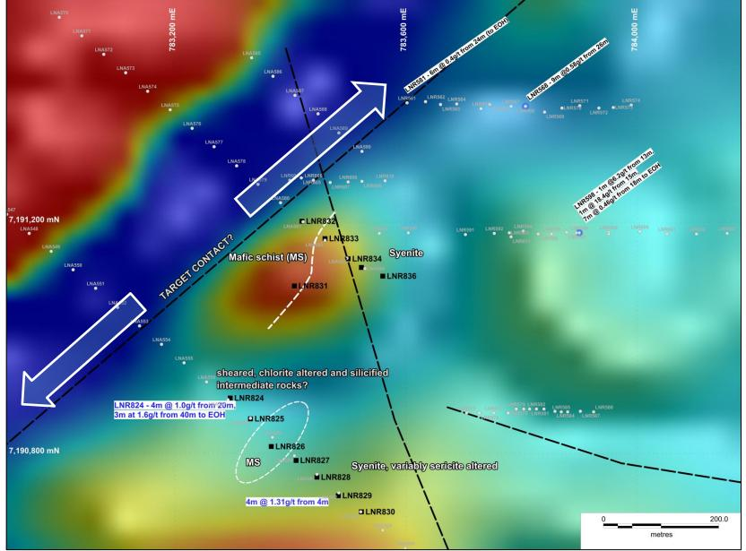
Figure 8 Brumby - drill collar plan, showing significant assay results (blue text), pre-existing drill collars and interpreted major structures on aeromagnetic (TMI) image (MGA94).
