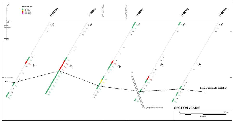
Figure 6 Contessa drill cross-section 29840E, looking northwest (showing gold assays greater than 10ppb Au).
