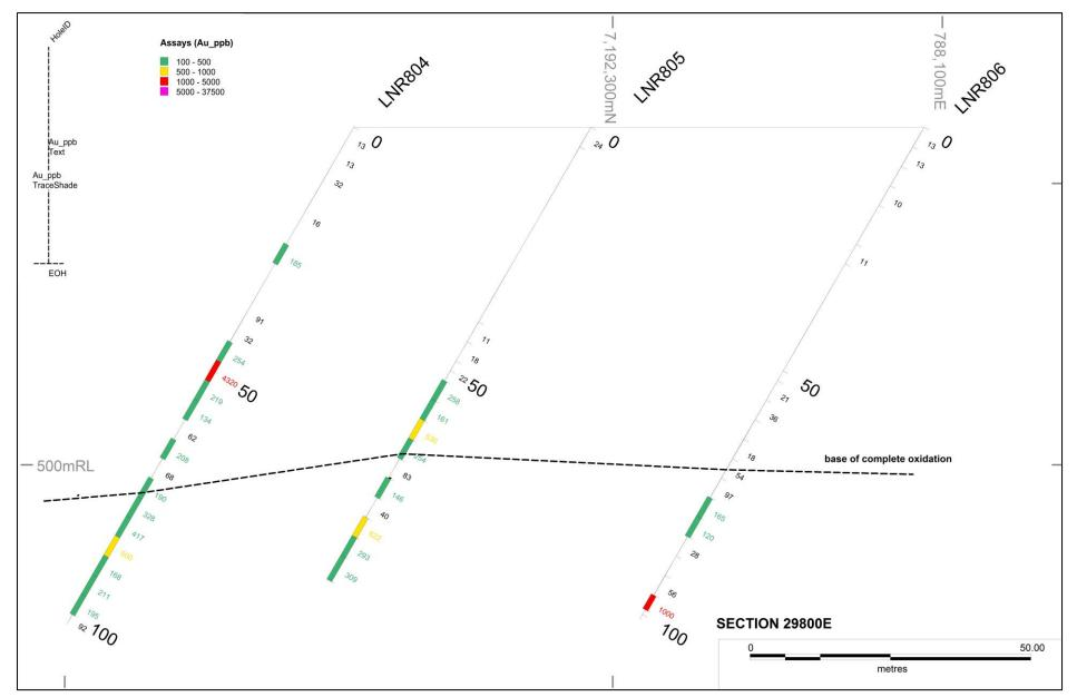
Figure 5 Contessa drill cross-section 29800E looking northwest (310 degrees) (gold assays greater than 10ppb Au).
