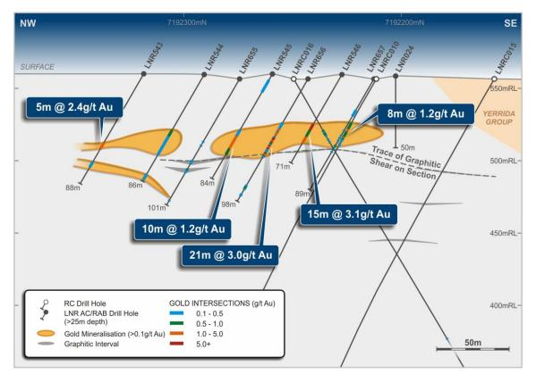
Figure 2 Contessa drill section 69700N, showing trace of graphitic interval and its relationship to mineralisation (graphitic interval is interpreted to dip into or out of the page, i.e. to northeast or southwest).
