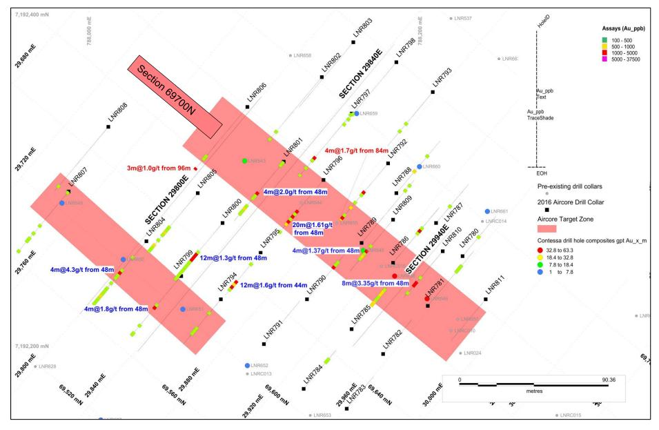
Figure 3 Contessa drill plan showing assay results and significant intersections (blue text) with transition zone intersections in red (MGA94, with local grid north at 40 degrees magnetic).
