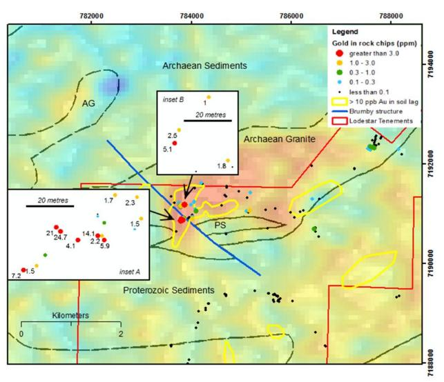
Figure 2 Brumby Prospect - Rock sample locations overlain on potassium radiometric image
