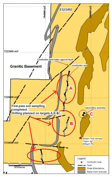
Figure 2 E52/2492 - Marymia late-time VTEM conductors shown on aeromagnetic image(TMI first vertical derivative).
