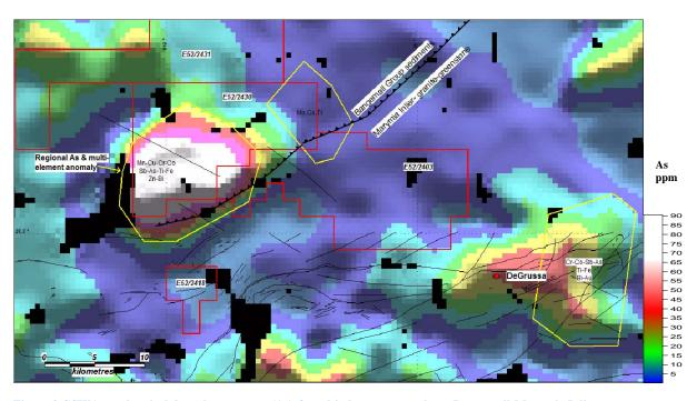
Figure 3 GSWA geochemical data shows strong (As) & multi-element anomaly on Bangemall-Marymia Inlier contact and intersecting NW trending structures. Note As & multi-element anomaly developed adjacent to the DeGrussa Cu-Au deposit. Grid MGA94 Zone 50
