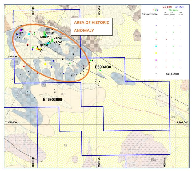
Figure 2 Rock sampling 95th percentile Cu-Pb-Zn distribution in relation to Jubilee Gold Mines NL RC drilling (NRC01 to NRC07). Background Rhodes (3147) 1:100 000 GSWA geology (MGA94 Zone 51).
