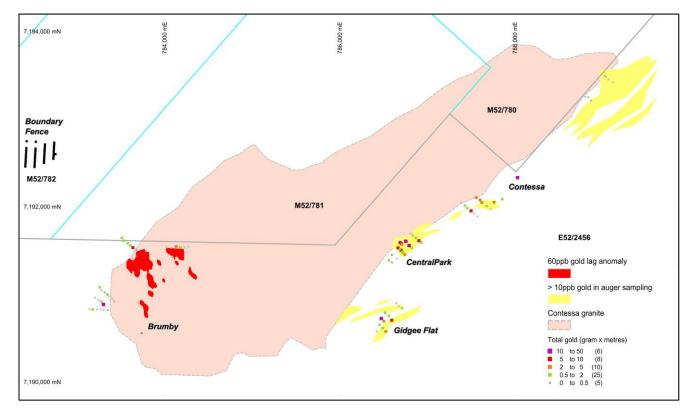
Figure 2 Drill hole location plan showing prospects, surface gold anomalies and colour coding total gold in each drill hole (grams per tonne of intersection x thickness of intersection).
