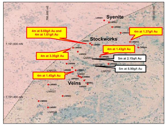
Figure 7 Central Park drilling showing significant intersections.
