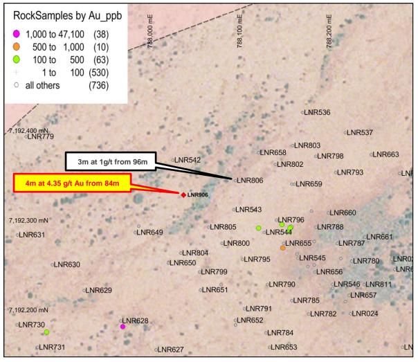
Figure 3 Bedrock gold target in LNR806 and LNR906 showing end of hole intercepts in mineralisation. Significant intersections from recent drilling shown in yellow/red boxes and previous intersections with black/white boxes. Red collars are recent drill holes.
