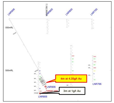
Figure 4 Cross section looking northeast showing relative intersections in LNR806 and LNR906.
