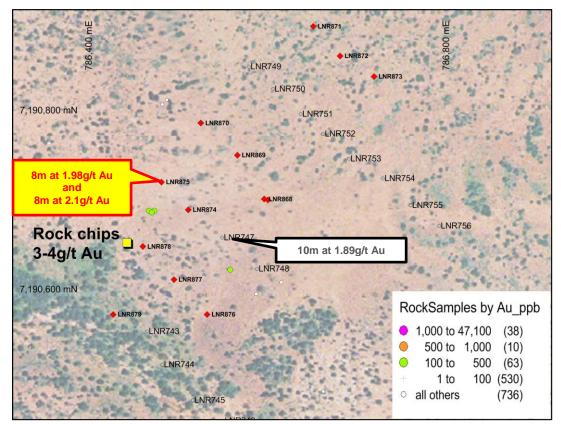
Figure 6 Gidgee Flat drilling showing significant intersections.
