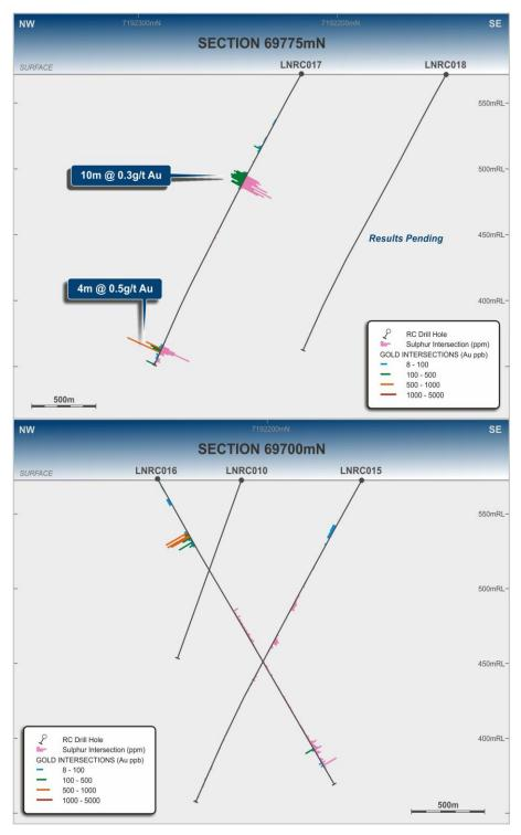
Figure 1 Cross-section views showing gold intercepts and relative sulphur (pyrite) abundance.
