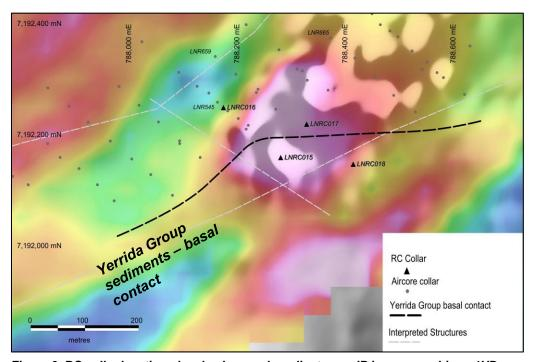
Figure 3. RC collar location plan, background gradient array IP image over hi-res 1VD magnetic image. MGA94 Zone 50.
