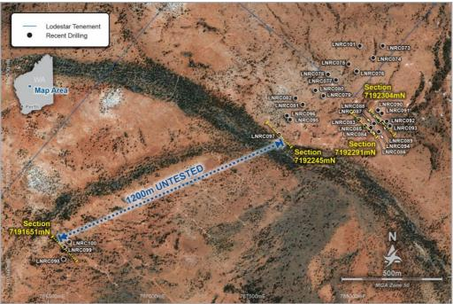
Figure 1 Drill collar plan.
