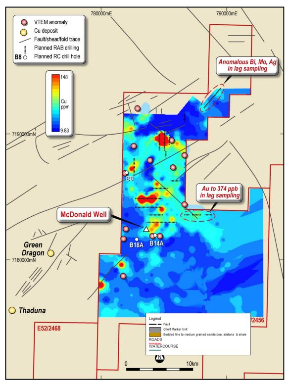
Figure 2 Planned drill program, McDonald Well showing copper distribution
