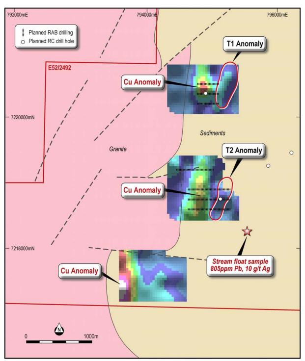
Figure 3 Planned drill program, Transformer prospect
