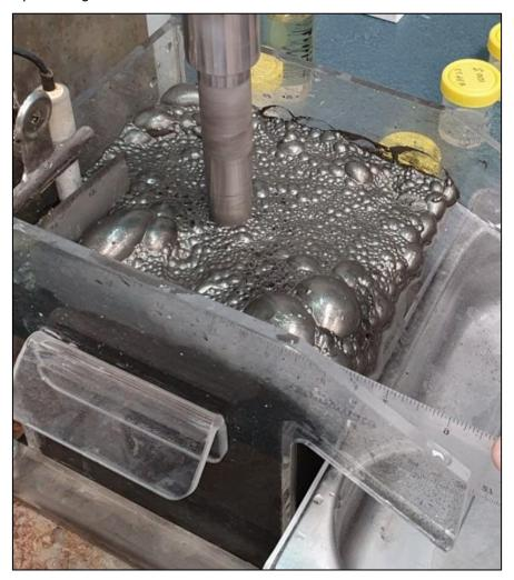
Figure 1 – Nickel concentrate (>13% Ni) produced during testwork on the high-grade massive nickel sulphides from Sample 3 (source: internal report from Strategic Metallurgy)
