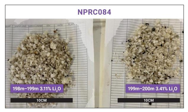
Image 1 - NPRC084 Drill Chips
