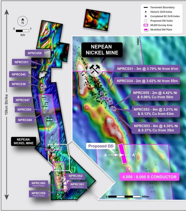
Figure 1 - Plan map of the Nepean Nickel Project showing EM conductor relative to aeromagnetics to the south of the historic Nepean nickel mine
