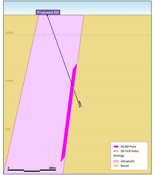
Figure 2 - Cross-section A - A' (see Figure 1) showing proposed diamond drill-hole and EM conductor in relation to the modelled ultramafic unit and interpreted footwall contact
