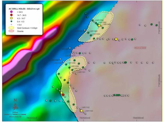
Figure 8 Brumby drill collar plan showing the distribution of gold anomalies on the granite contact (1VD RTP aeromagnetic image).
