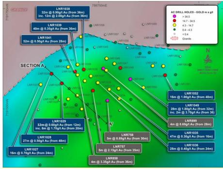
Figure 7 Central Park drill hole plan showing gold distribution and drill intersections (1VD RTP aeromagnetic image)
