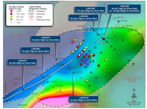
Figure 6 Gidgee Flat target contact, showing extent of aircore drilling (1VD RTP aeromagnetic image background)
