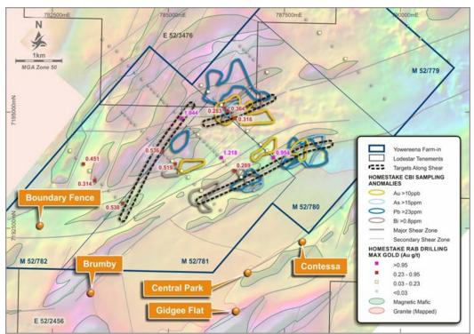
Figure 9 Multi-element geochemical anomalies and gold in historic aircore drilling on RTP aeromagnetic image.
