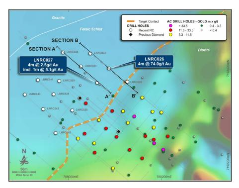
Figure 2 Contessa drill hole plan showing collar locations and supergene gold distribution in aircore drilling on background aeromagnetic image.
